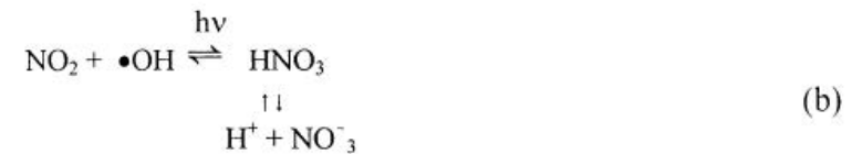
Fig. 12. Reaction networks for photocatalytic oxidation of nitric oxide over \text{TiO}_2 .
