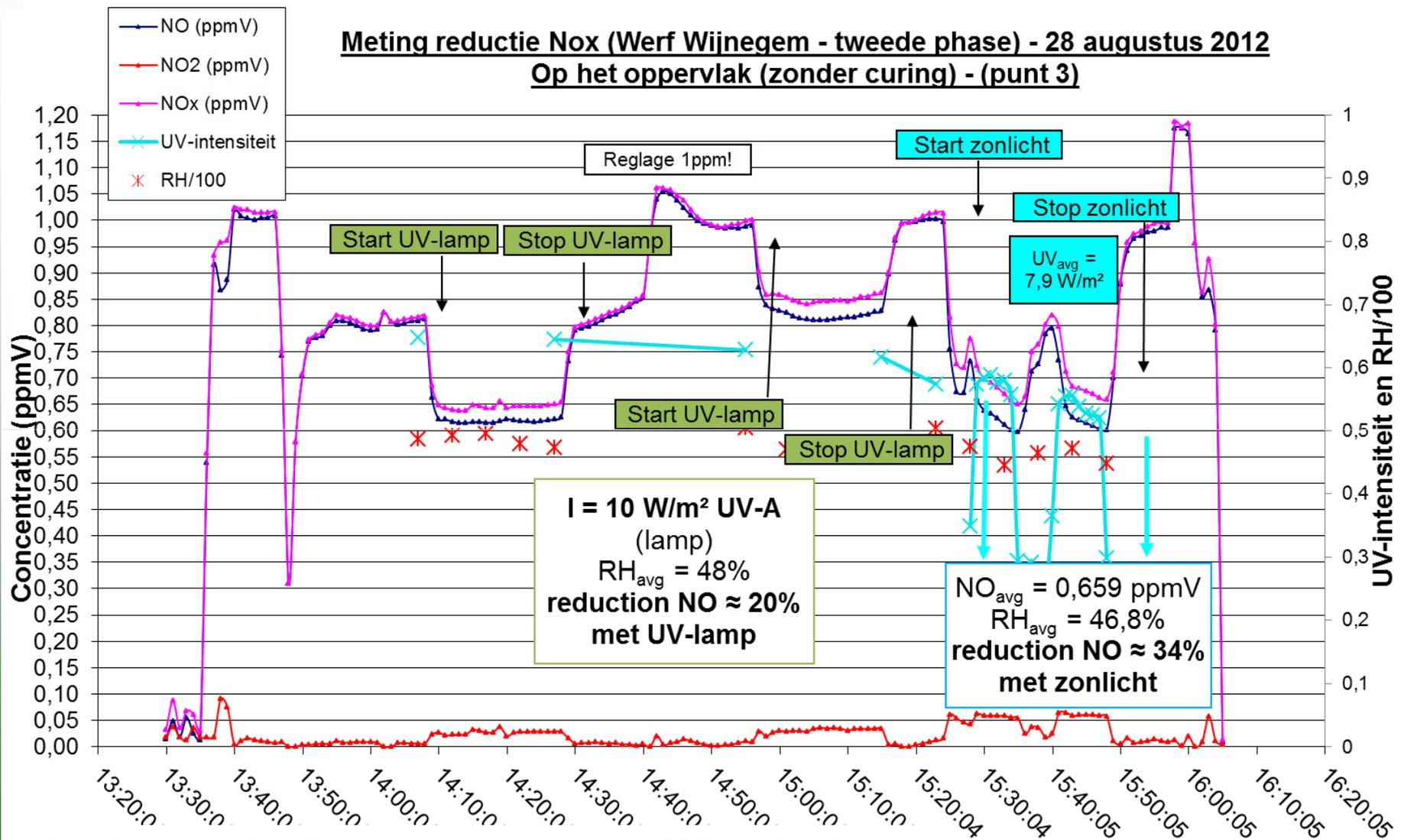
Reduced reduction: 34% versus 52% NO-reduction – durability? Pollution of the surface?
