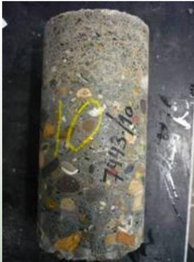
double layered concrete with recycled concrete aggregates in base layer and photocatalytic concrete in top layer on industrial zone “Den Hoek” in Wijnegem and in “Duwijck” in Lier, Belgium
