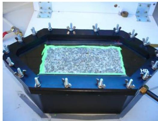
**Pre-treatment: rinsing with distilled water and drying overnight at laboratory conditions**
