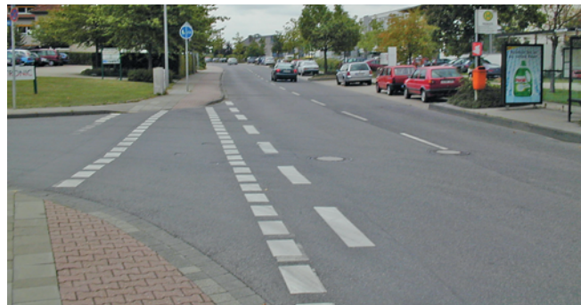
Road in a commercial area with a divided longitudinal parking lane, cycle traffic sharing the footway space, bus stop
