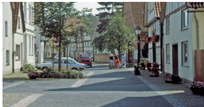
Village-style residential street with 'soft separation' and offset parking bays
