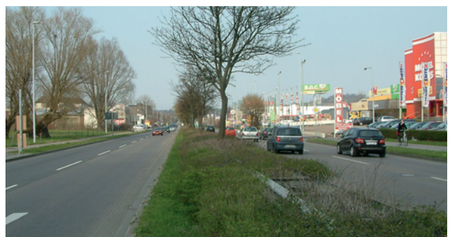
No frontage access road, central reservation with planting, also pedestrian and cycle paths on both sides within built-up areas
