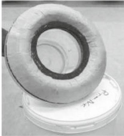
Figure 4: Sealing with bentonite beneath the base plate
