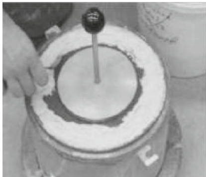
Figure 5: Applying the bentonite powder to the sample surface
