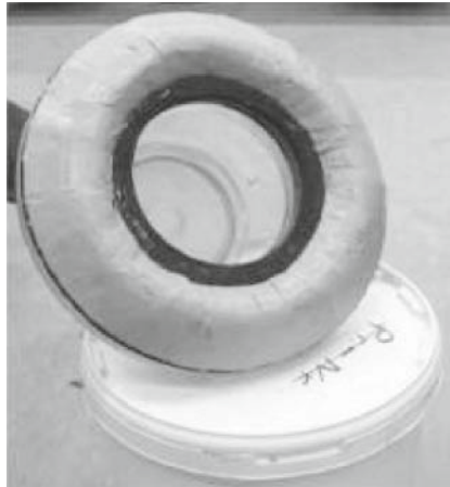
Figure 4: Sealing with bentonite beneath the base plate
