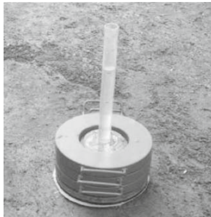
Figure 5: Modified vertical tube infiltrometer during in situ testing
