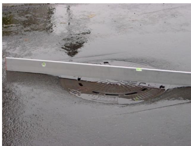
Figure 21: Checking the height of a manhole [7]
