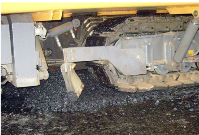
Figure 47: Paver track unit running over cold spilled asphalt mix [11]
