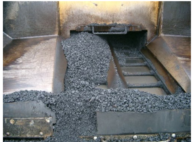
Figure 48: Material segregation and exposed tunnel due to hopper wings being folded too late [11]
