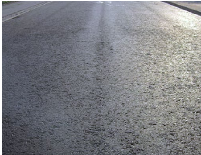
Figure 44: Segregation in an asphalt base course AC 32 T S due to inadequate distance between auger and screed tamper shield [11]
