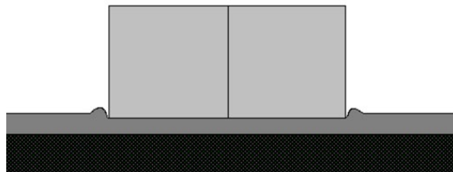
Figure 80: Bulging adjacent to the drum [38]
